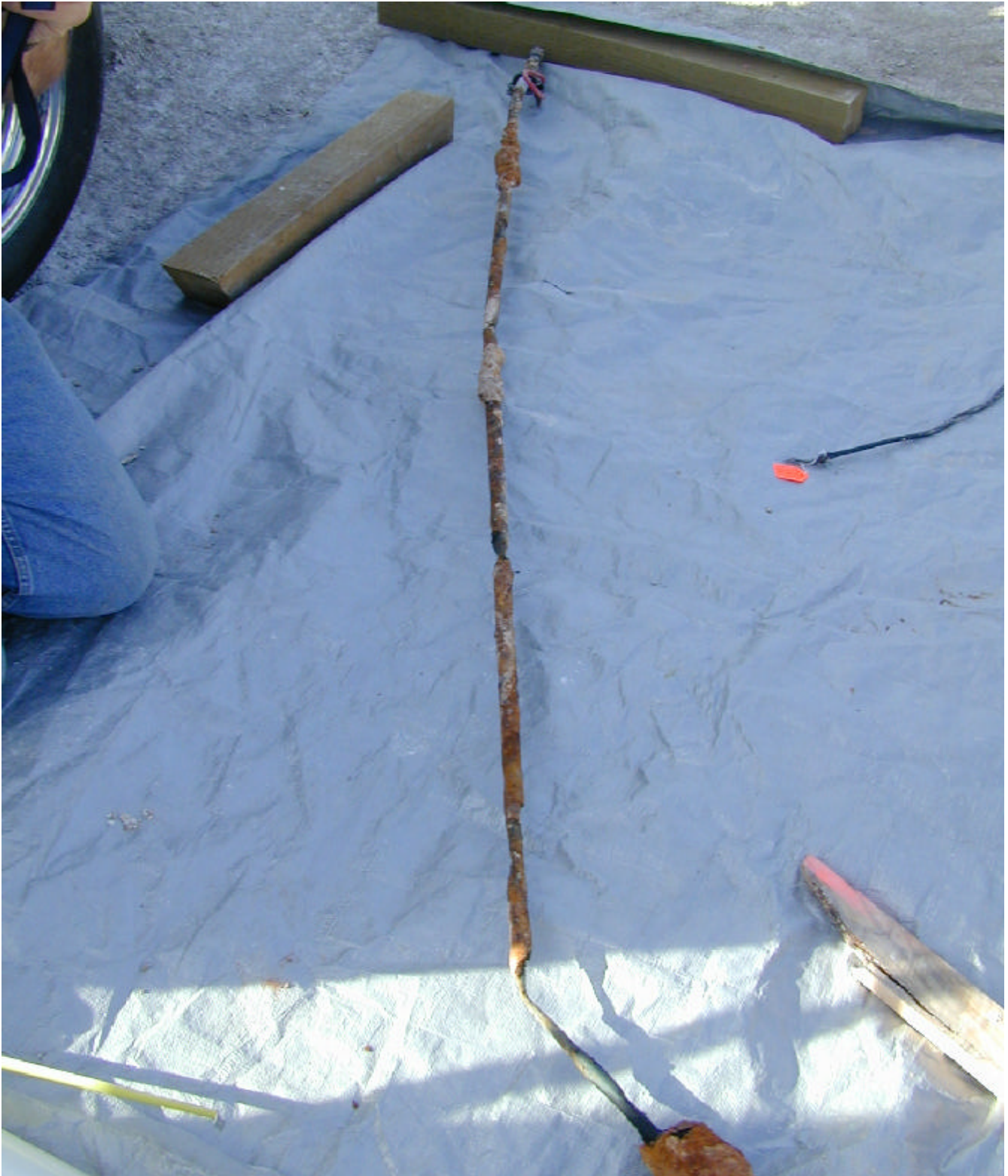
Figure 1. \frac{3}{4} " x 10' galvanized rod removed after 10 years (Pawnee Site).
